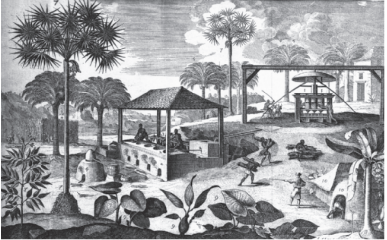
MAKING MOLASSES IN BARBADOS African slaves, who constituted the vast majority of the population of the flourishing sugar-producing island of Barbados, work here in a sugar mill grinding sugarcane and then boiling it to produce refined sugar, molasses, and—after a later distillation process not pictured here—rum. ( Arents Collections, Rare Books Division, New York Public Library, Astor, Lenox and Tilden Foundations )
